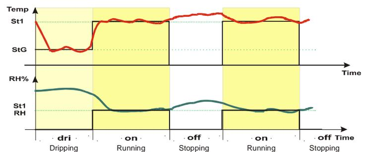
The diagrams displays a typical maturing cycle with the starting dripping phase.
