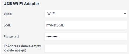
Configuration changes can be made by the user after accessing the user interface from the System→Settings→Network menu.
