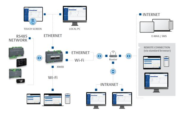
Before connecting the XWEB to the network, check that the IP address you wish to use for the XWEB is actually free and therefore usable. You could perform a PING to that address and if at least one reply is received at the PING, the address must be changed as it is already used.
