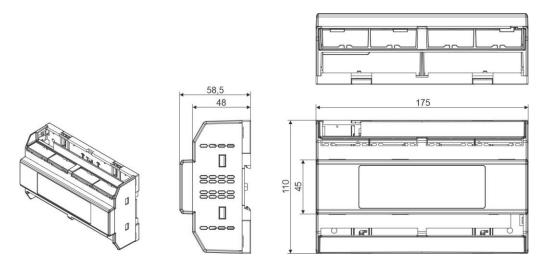
XWEB is DIN Rail mounting compatible. Snap the orange tabs on the back of the unit to the down position to fasten. If not using the DIN Rail mounting option, fasten to the mounting surface using the openings in the mounting tabs.
