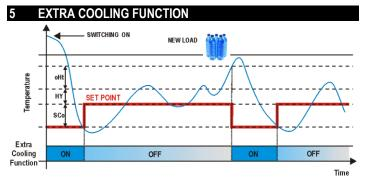
The SUPER-COOLING function is active when the room temperature measured from the probe 1 goes over the SET+oHt+HY value. In this case, a special set-point value, lower than the normal SET value, will be enabled. As soon as the room temperature reaches the SET-SCo value, the compressor will be stopped and the normal regulation will restart. N.B.: super-cooling function is disabled when SCo=0.
