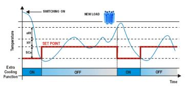
The SUPER-COOLING function is active when the room temperature measured from the probe 1 goes over the SET+oHt+HY value. In this case, a special set-point value, lower than the normal SET value, will be enabled. As soon as the room temperature reaches the SET-SCo value, the compressor will be stopped and the normal regulation will restart. N.B.: super-cooling function is disabled when SCo=0.
