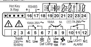
**Supply: 110Vac:** connect to terminals 2-3. oA3= configurable relay
