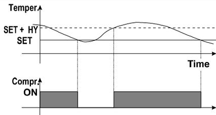
For each section, the regulation is performed according to the temperature measured by its own thermostat probe with a positive differential from the set point.
