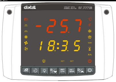
To display and modify target temperature set point. (SET TEMP) for the running (St1) and the dripping (StG) phase.
