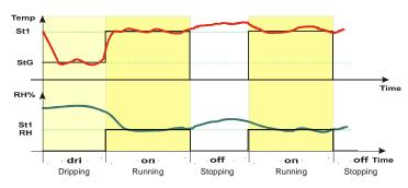
The diagrams displays a typical maturing cycle with the starting dripping phase. DRIPPING PHASE lasts for the "dri" time, without humidity control, temperature set is SETG RUNNING PHASE lasts for the "on" time, both temperature and humidity are controlled.
