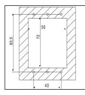
Keyboard **VC660** shall be mounted on vertical panel, in a 72x56 mm hole, and fixed using screws  $\varnothing$  3 x 2mm. To obtain an IP65 protection grade use the front panel rubber gasket (mod. RGW-V).
