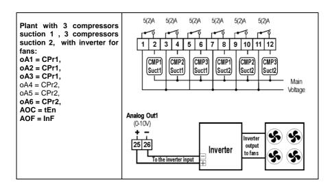
**CtyP** Compressor type: it sets if compressors have the same power (homogeneous) or not.
