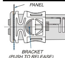
Instrument XA100C shall be mounted on vertical panel, in a 29x71 mm hole, and fixed using the special brackets supplied. To obtain an IP65 protection grade use the front panel rubber gasket (mod. RG-C).
