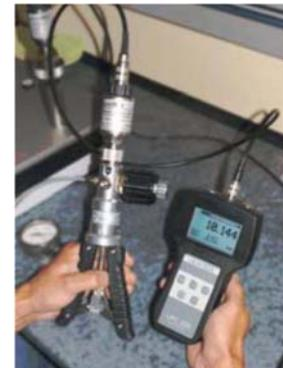
Using the optional **LPC-Cal** software, the logged data, stored in the **LR-Cal** LPC 200, can be transferred to a PC via a USB connection, where it can be stored in an Excel® file for documentation and further evaluation. In addition, **LPC-Cal** offers the possibility of PC-supported calibration of pressure measuring instruments using the **LR-Cal** LPC 200.
