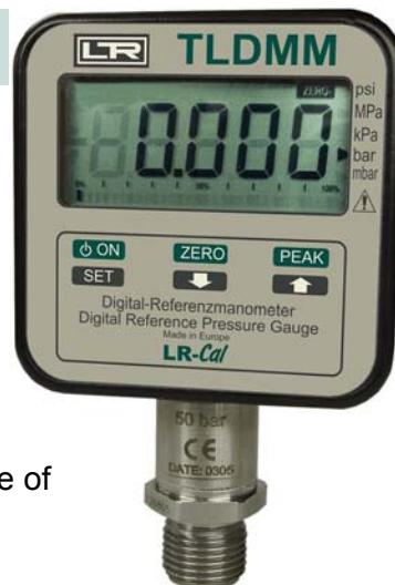
The **TLDMM** is a microprocessor based digital pressure gauge, made of particularly high long-term stable analogue section and an 16 bit A/D converter which ensure 65,000 internal divisions. These features, together with a 0.05% accuracy class, make it ideal as a laboratory instrument: in fact the **TLDMM** is proposed as a first line sample for Calibration Laboratories and is provided with a S.I.T. calibration certificate, traceable to international standard.
