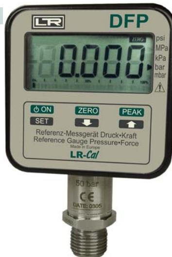
The Digital Reference Pressure Gauge **DFP** has internal batteries with 1 year autonomy, also guaranteed by the Auto-PowerOff function, which activates if no measurement changes are detected in the previous 30 minutes (adjustable).
