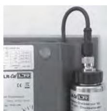
Reference pressure sensor **LR-Cal** LPC-S externally with optional extension cable connected to **LR-Cal** LPC 300
