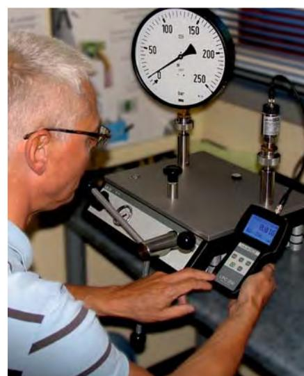
**Digital Reference Pressure Indicator Type TLDMM
