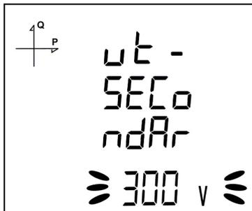
1. Enter the secondary value of your VT by using SET and UP/DOWN buttons.
