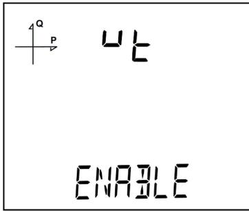
1. By using UP/DOWN buttons, select Enable or Disable indicating whether you use a voltage transformer on your system.
