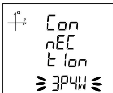
1. By using UP/DOWN buttons, select your network connection type as 3P4W, 3P3W, ARON, 3P4W Balanced or 3P3W Balanced.
