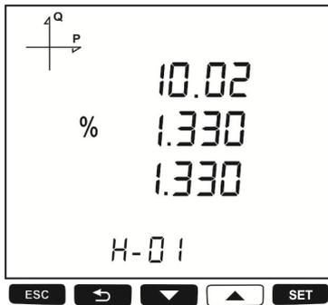
Current screen is displayed when “V I F” button is pressed. When THD H button is pressed at this point, following screens are displayed.
