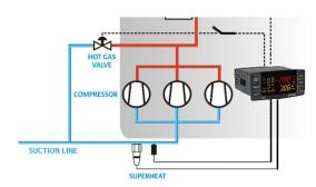
To detect the suction superheat an auxiliary probe among P4 (term. 13-14) has to be set as superheat temperature probe.
