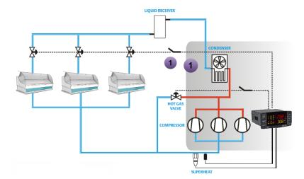
To enable this function set one relay by the parameters **oA2** or **oA4** or **oA5**, as flood protection, El **oA4 = Liq,** and then connect it to the external device that blocks the cabinet injection.
