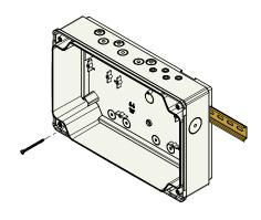
DIN Rail mounting allows an efficient alignment of multiple controllers. This is useful in case of applications where there are several cold rooms.
