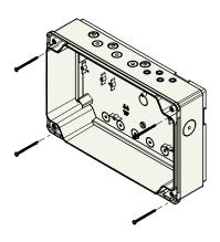
4 screws, with pre-formed posts and in 4 corners separated by gasket from the inner part, allow you to attach the controller quickly and safely to the wall.
