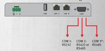
\*\* CAB150 splitter cable provides the connectivity for the three serial ports.
